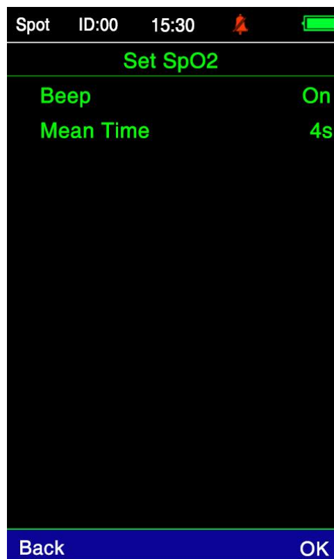
Figure 3-10 Blood oxygen setup menu
