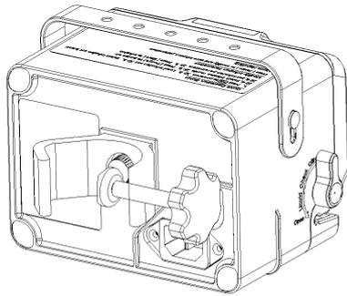
1. Turn counterclockwise to loosen the pole clamp until an IV stand can be inserted in.
