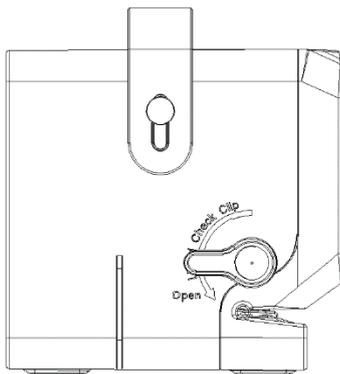
2. Rotate the Liquid Check Clip backward 90° to open.
