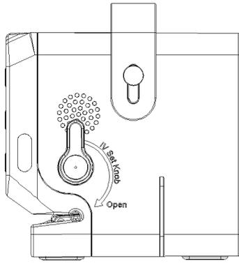
4. Rotate the IV Set Knob forward to close position, the **[Select Brand]** interface will pop up, indicating that the tube is installed correctly.
