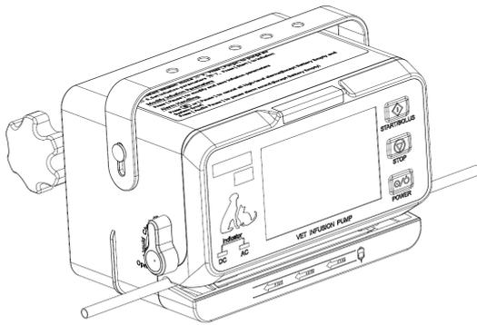
5. Install IV set completely, if the **[Select Brand]** interface will not pop up, the tube needs to be re-installed.
