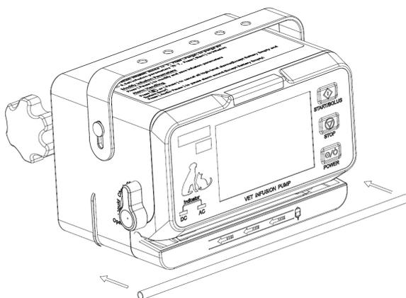
3. Straighten the IV set and horizontally place into the tube slot, and move back and forth in the tube slot several times to ensure that the IV set installation is straight and correct.
