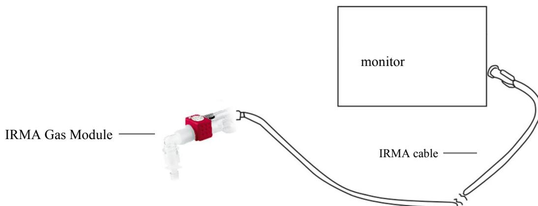
Figure 15-1 IRMA gas module connection
