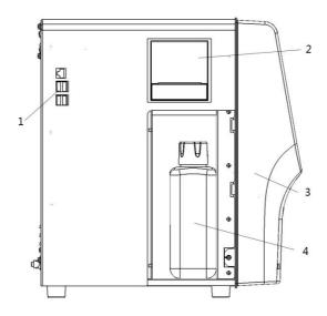
Figure 2-3 Left view of the analyzer (left door open)
