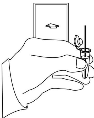
3. Press the aspirate key and add the diluent (180 $\mu$ L at a time)
