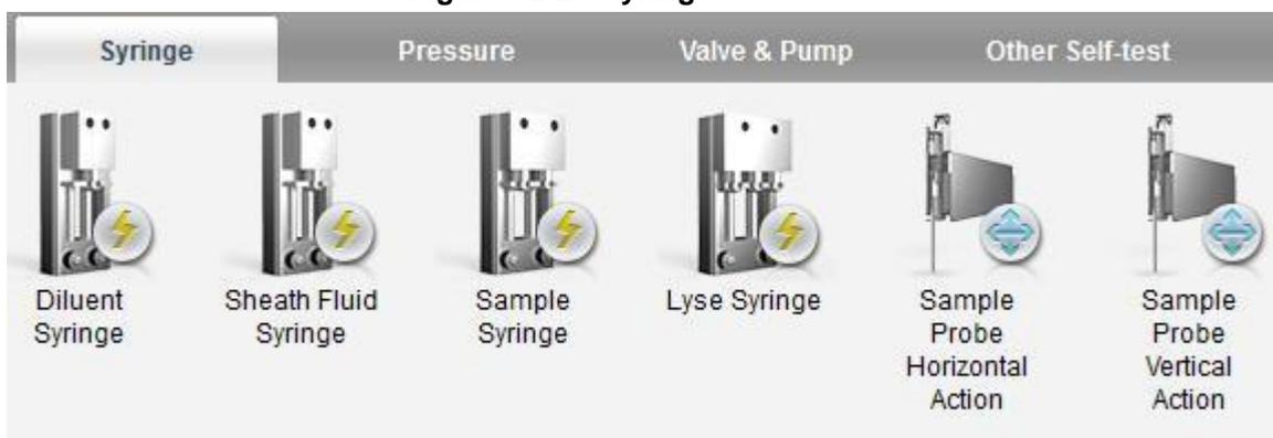
2. Double click the part that needs to be tested, e.g. **Diluent syringe**, and wait for the self-inspection results.
