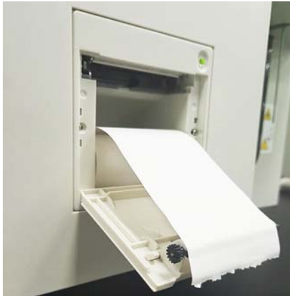
Figure 2-9 Installing Thermal Paper (2)
